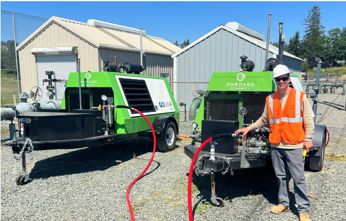
Figure 9. Multiple units can be used for larger evacuation projects.
