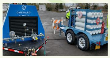
The GoFLO compressor is delivered on a trailer frame with lights and brakes so that it can be licensed in most states as mobile equipment. This mounting makes the GoFLO easy to be installed and re-positioned as necessary.
